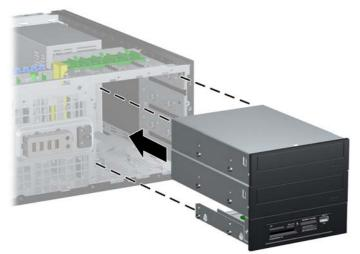
Figure 5-58 Installing a Drive in the Desktop Configuration
